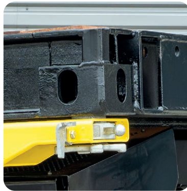
The CROCO40 is fitted with secure container fasteners.
