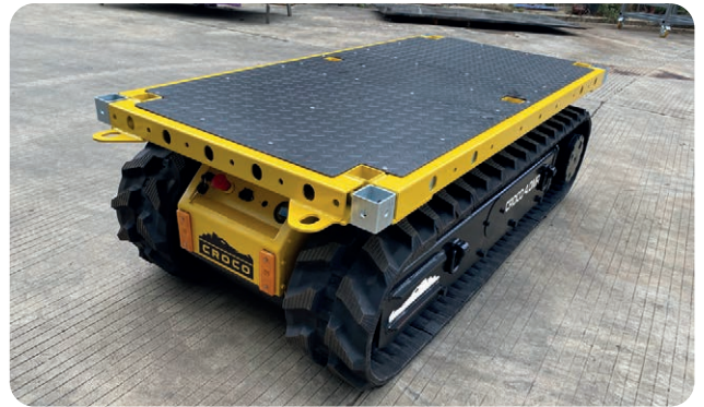
The CROCO4.0 is a low profile carrier for moving heavy goods over rough ground.
