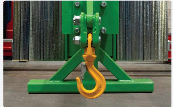
The stand helps to protect the overhang beam when storing or transporting
