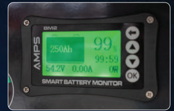
The clear to read LCD screen displays the remaining battery percentage, current voltage, live current draw, remaining run time and power consumption in Watts
