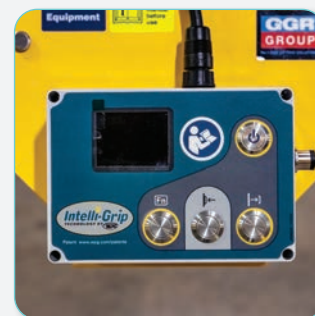
The Intelli-Grip technology monitors vacuum lifters in real-time.
