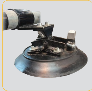
Flexible pads and swivel arms to attach to convex or concave loads
