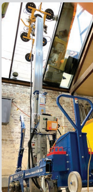
The GML800+ can be used with its own optional glass vacuum lifter with radio remote for total control when glazing at height. The maximum capacity is reduced if using the VGL98 Glass Vacuum Lifter to 500kg.
