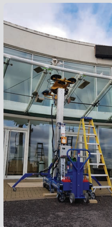
The GML800+ can be used with its own optional glass vacuum lifter with radio remote for total control when glazing at height. The maximum capacity is reduced if using the VGL98 Glass Vacuum Lifter to 500kg.
