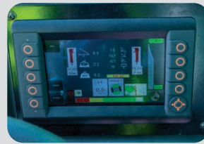
The MC350 Pick & Carry Crane comes with a full colour SLI system
