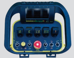
The MC350 Pick & Carry Crane can be fully controlled via radio remote with digital screen
