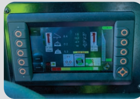
The MC250 Pick & Carry Crane comes with a full colour SLI system
