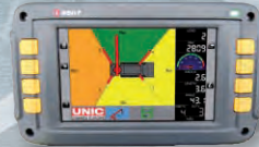
Variable Footprint safe load indicator
