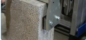
The other jaw is lined with a replaceable rubber pad to ensure the grip on the stone being lifted is secure.
