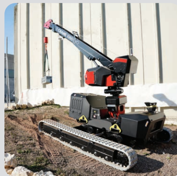
The T-Crane 1060 can handle gradients of up to 25° with ease.
