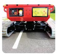
The deck can be moved between three heights for extra ground clearance.
