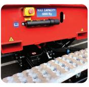
Forklift and lifting points are included to move the Tracked Leveller 5.5 on transport or to harder to reach areas.
