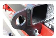
The lifting points on both the bed and crane platform means the crane can easily be removed to use the Leveller as a trolley only.
