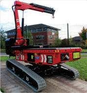
Able to pick up from the ground, lift loads onto it's own bed, track to the final location and install items over rough terrain makes the Tracked Leveller 5.5 with crane one of the most versatile machines on any work site.
