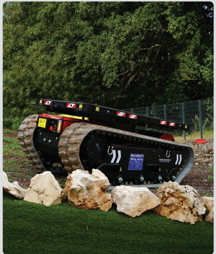
The ML 3.0 RT with wider tracks and a higher ground clearance is ideal for carrying heavy loads while traversing rougher terrain.
