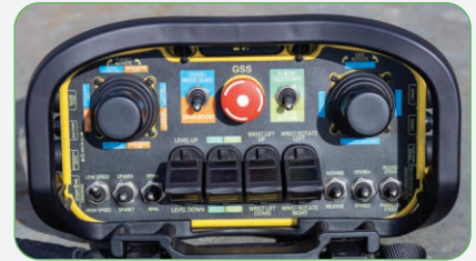
The Sky Robot 1500 is controlled by a high precision radio remote control
