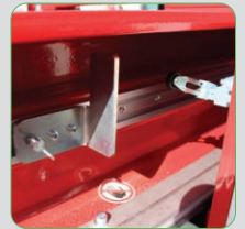
A moveable limit switch allows the operator the ability to stop the counterweight saddle from moving further back than determined.
