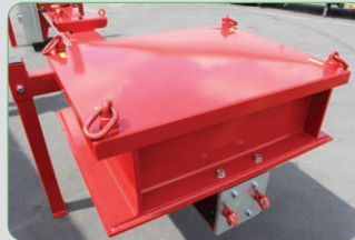
Featuring a removable counterweight, note the counterweight must be installed when using the corner lifter attachment. (Weight of removable counterweight: approx. 1500kg)
