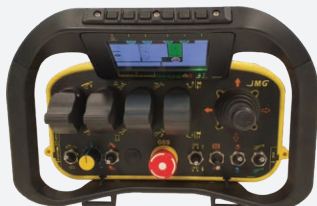
The MC32S is fully controlled by radio remote with digital feedback display
