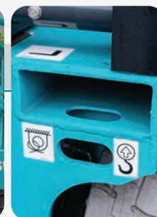
Lifting eyes are included for ease of transport or moving from level to level by crane.
