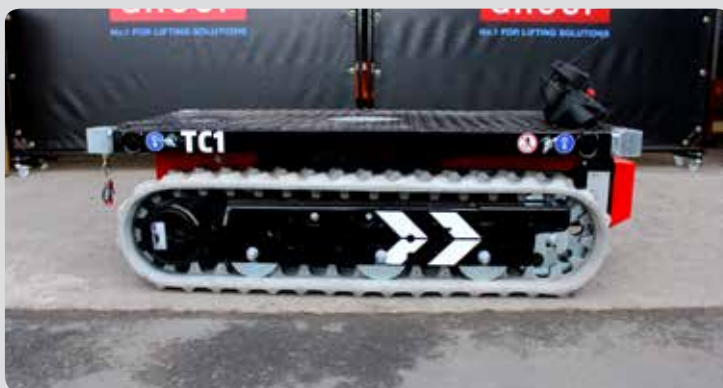
The tracks of the TC1 means it can be used to transport materials on uneven ground.
