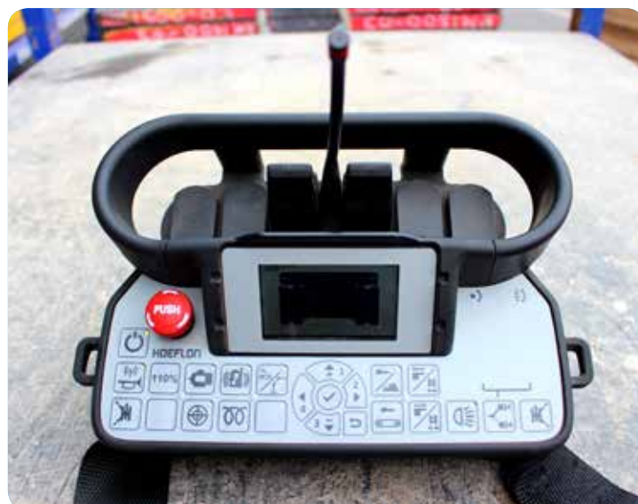
The TC1 Tracked Carrier is controlled by a radio remote control with digital feedback.
