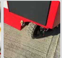
180° rear hydraulic steering for optimal control
