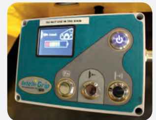
The Intelli-Grip technology monitors vacuum lifters in real-time.
