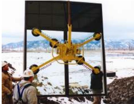
When temperatures rise above 40°C, the pumps and other components on all electrically powered lifters can over heat and stop working all together.
