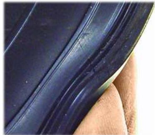
When releasing a load from the lifter, allow air to flow into the system as designed. Torn sealing edges not only increase the time it takes to attach a lifter or prevent it from reaching full vacuum, but also pose a danger for unexpected release of the load.
